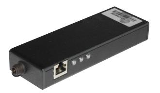
over the DDU, data is wirelessly transmitted back to the unit. The powerful onboard processors determine the 'health' of the door. This data is transmitted over a network to a database for storage and analysis, where historical trends can be plotted. From the database a detailed profile of the door behaviour is obtained, including velocity curves at each stage of an open or close process.
