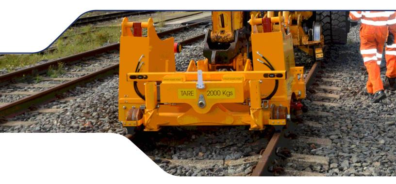
Remove clips at up to 2.5 miles of track per hour Simple, safe, efficient and proven technology Automatic system to prevent damage to ties Fully approved by Network Rail
