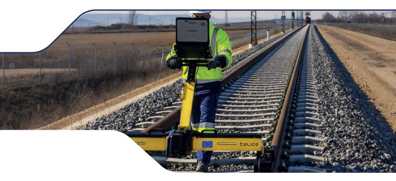
Reliable, low cost geometry measurement solution Real-time, actionable information Automatic measurement - height and stagger Foldable design, easy to transport
